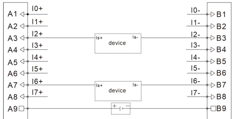
Note: A9 and B9 are external power input interfaces.
