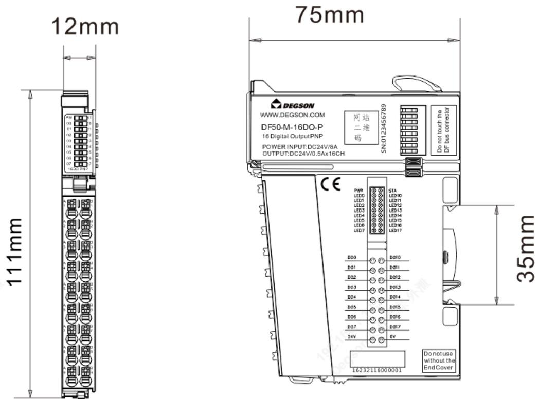
16 channel digital output module /24VDC/PNP
