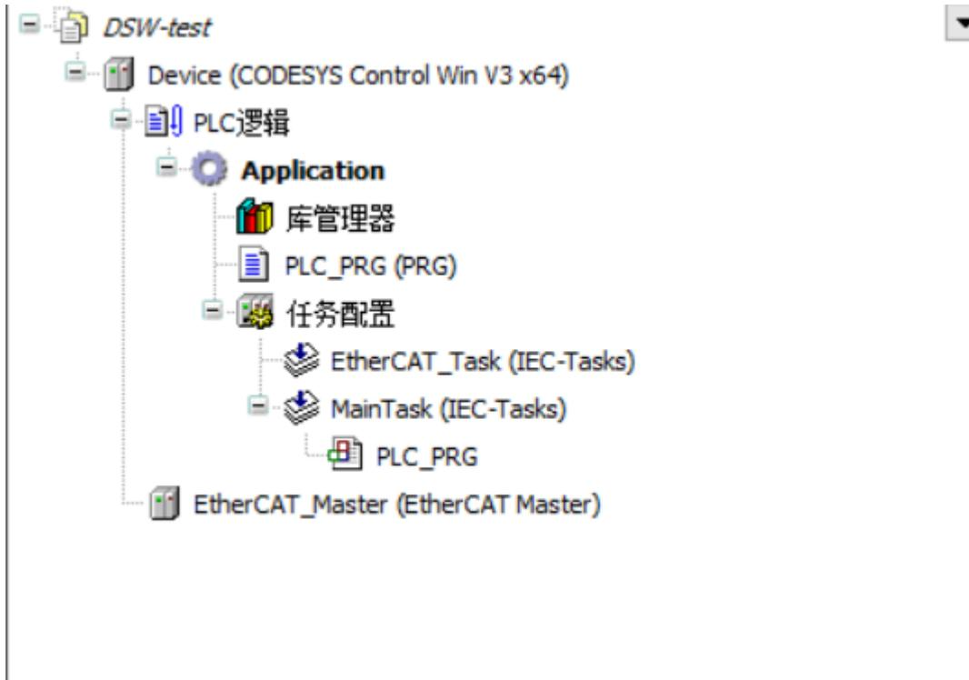
Log in to the downloader and
