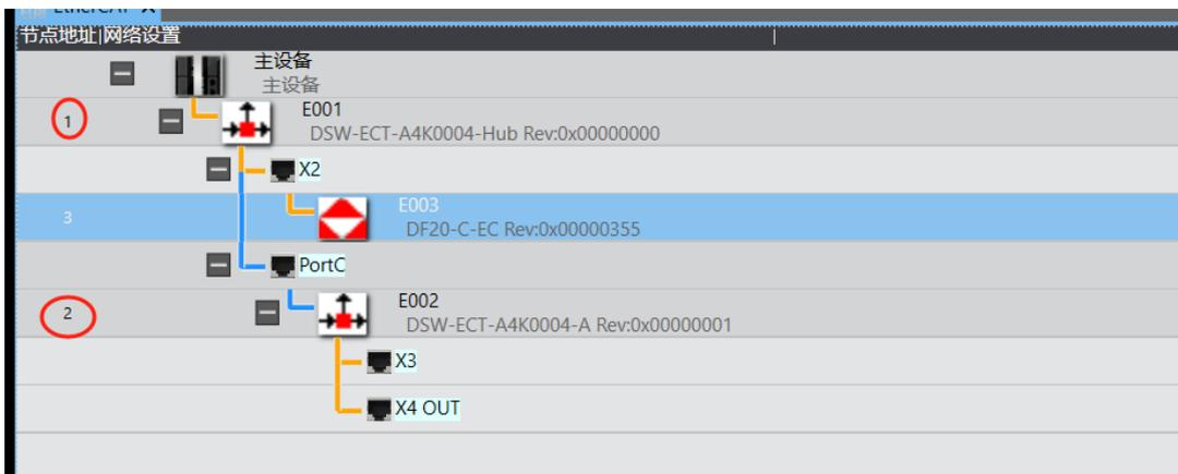
Add the module to the corresponding network interface, configure the "Node Address", and then download it to the controller:
