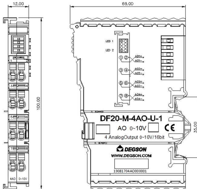
◆ **4 channel Analog output /voltage type / $\pm 10V$ , 0~10V (DF20-M-4AO-U-4)**
